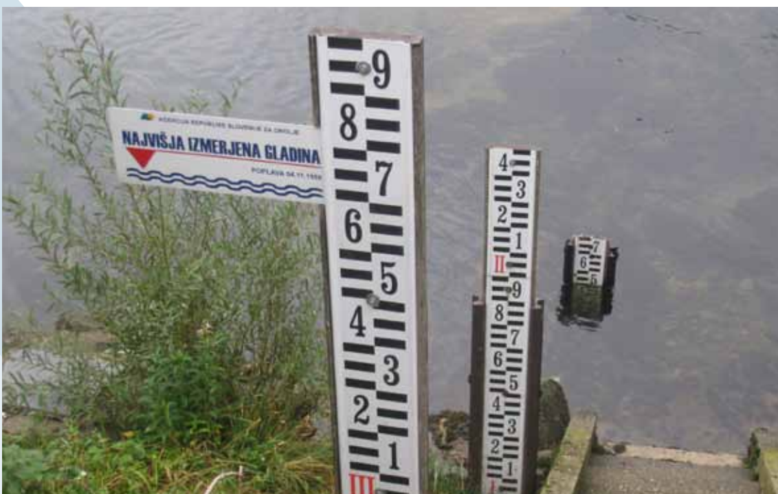
Hidrološko merilno mesto za spremljanje višine vodotoka Hydrological measuring station for the monitoring of the watercourse-level
