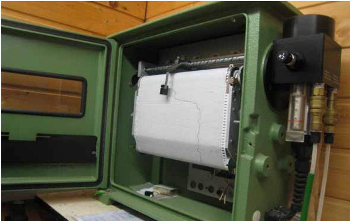
Prej: Limnigraf za merjenje gladine vode Before: Limnigraph for the recording of water-level
