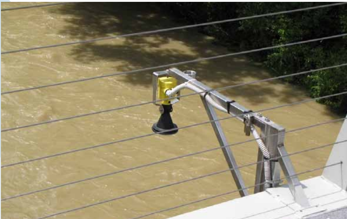
Potem: Radarsko merjenje gladine vode Afterwards: Radar-based measurement of the water level
